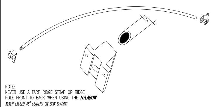
UNBREAKABRACKETS MUST BE USED WHEN INSTALLING THE NYLABOW
